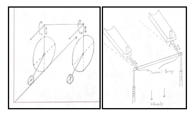
Figure 3. Concept 3 general view on the left and top section view on the right.
